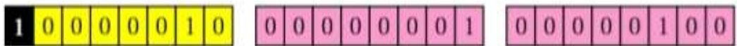
b. The yellow part defines the length of the length (2 bytes); the pink bytes define the length (260 bytes)
